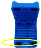
3. Cut the cable jacket by maintaining pressure on the cable cutter, pull the tool in the direction indicated. The cable jacket is cut at the top and bottom
