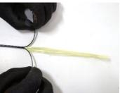
5. Using cutting pliers, remove the two sheath halves
